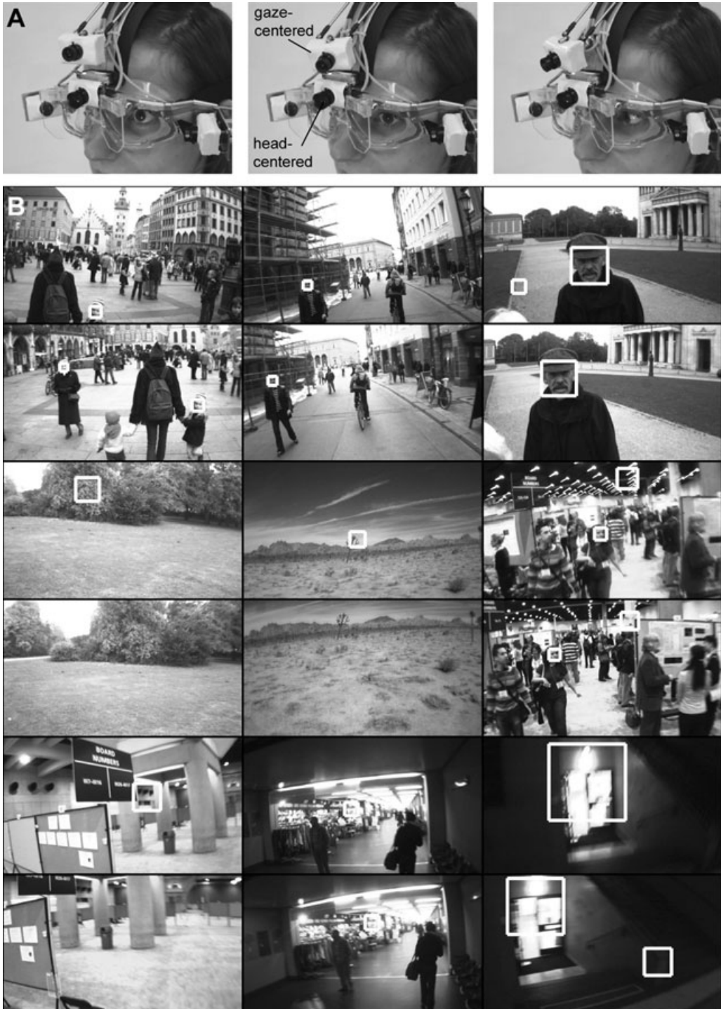
Figure 1. (A) The EyeSeeCam recording setup. The head camera is fixed in head coordinates, while the pivotable-gaze camera is automatically aligned to the direction of gaze in real-time. (Adapted from Schumann et al. 15 ) (B) Representative frame of each environment (environment (1), upper left; (3), upper right; (9), lower right). Top: Gaze-centered recordings. Bottom: head-centered recordings. White boxes denote face detections.
